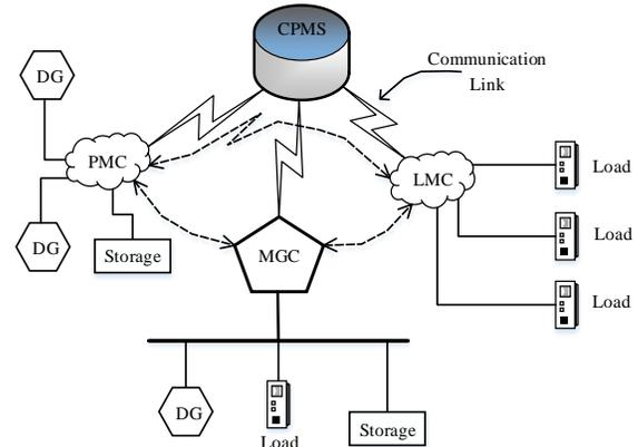
Figure 1. Hierarchical control structure of integrated microgrid
