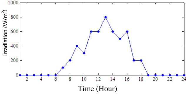
Figure 8. The input irradiation data for simulated model
