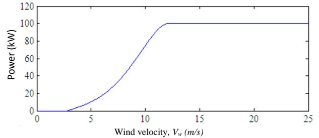
**Figure 6.** Power curve of a 100 kW turbine
