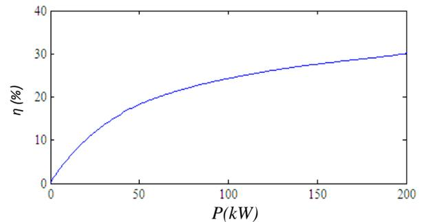
Figure 4. Output power vs. efficiency curve of MTG
